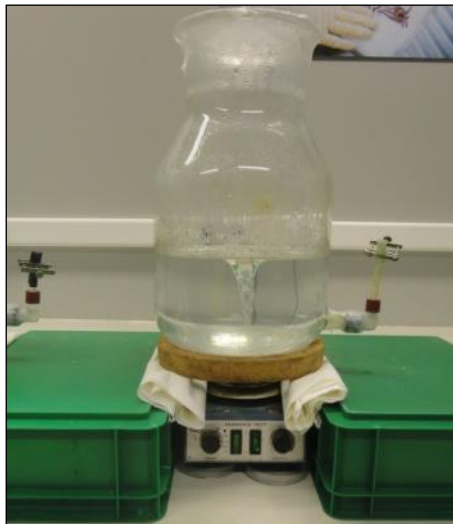
Figure 7. Visual presentation of the test set-up in order to prepare the WAF.
