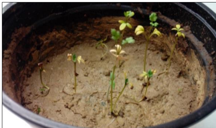
Figure 35. Chlorosis and stem and leaf deformation - Series 2 (last day of the test - two weeks of growth) (Ecotoxicity test OECD 208).
