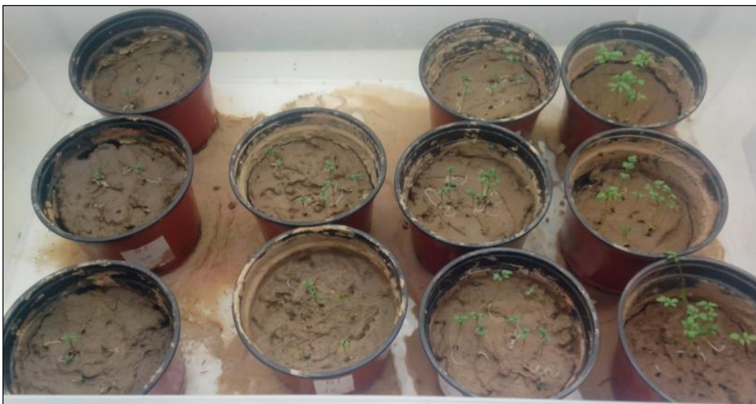
Figure 41. Growth of cress plants (OECD 208) after 7 days in pots with sunflower oil (three month from the test set-up).
