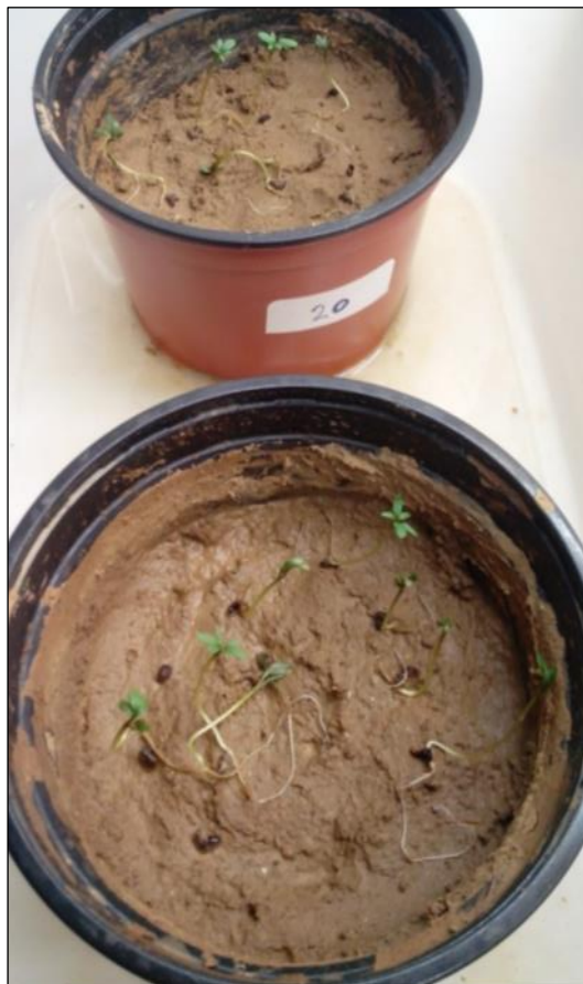
Figure 36. Chlorosis and stem and leaf deformation- Series 3 (last day of the test- two weeks of growth) (Ecotoxicity test OECD 208).
