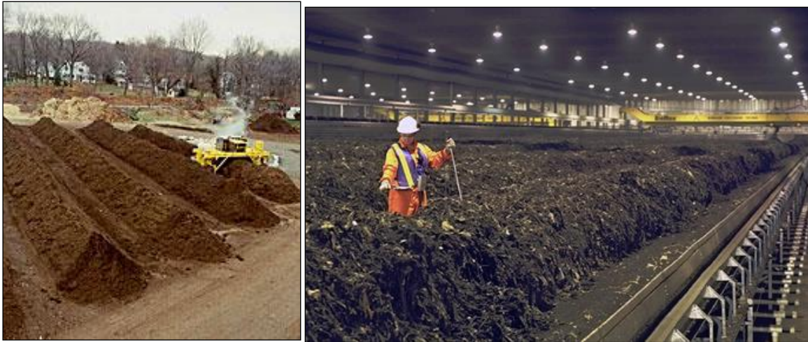
Figure 3. Open air windrow system (left) and a closed hall windrow system (right).
